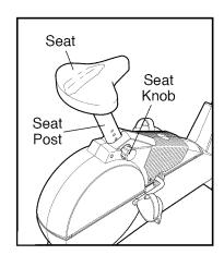
loosen it (if the knob is not loosened enough, it may scratch the seat post). Next, pull the knob, slide the seat post to the desired height, and then release the knob. Move the seat post up and down slightly until the pin on the knob snaps into one of the holes in the seat post. Then, turn the knob clockwise until it is tight.
