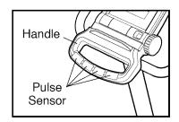
To use the pulse sensor, hold the handle on the console, with your right palm covering the two right contacts and your left palm covering the two left contacts. Avoid moving your hands. When your pulse is detected, the heart-shaped indicator in the display will flash each time your heart beats and two dashes (--) will appear. After a moment, your heart rate will be shown. For the most accurate heart rate reading, continue to hold the handgrips for about 15 seconds.
