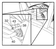
indicated M4 x 16mm Screw (32). Slide the Reed Switch slightly closer to or away from the Magnet. Retighten the Screw. Turn the Crank Arm for a moment. Repeat until the console displays correct feedback. When the Reed Switch is correctly adjusted, reattach the left side shield, the side shield cover, and the left pedal.
