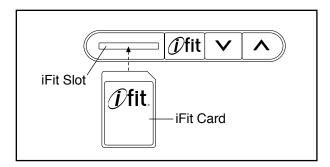
Select the desired workout on the iFit card by pressing the increase and decrease buttons next to the iFit slot. The duration of the workout will appear in the left display, the maximum resistance level for the workout will flash in the center display, and the number of the workout will appear in the right display.
