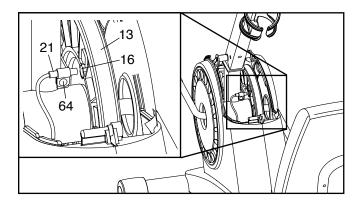
Slide the Reed Switch (21) slightly closer to or away from the Pulley Magnet (16), and then retighten the M4 x 15mm Screw (64). Turn the Pulley (13) for a moment. Repeat these actions until the console displays correct feedback.
