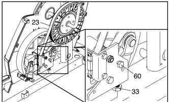
When the Drive Belt (23) is tight, tighten the M6 x 20mm Hex Screw (60).
