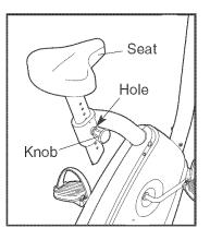
slide the seat post up or down, and align one of the adjustment holes in the seat post with the indicated hole in the seat frame. Insert the seat knob into the seat frame and the seat post, and turn the knob clockwise until it is tight. Make sure that the seat knob is inserted through one of the adjustment holes in the seat post.
