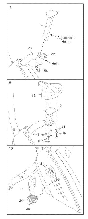
11. Make sure that all parts are properly tightened before you use the exercise cycle. Note: After assembly is completed, some extra parts may be left over. Place a mat beneath the exercise cycle to protect the floor.
