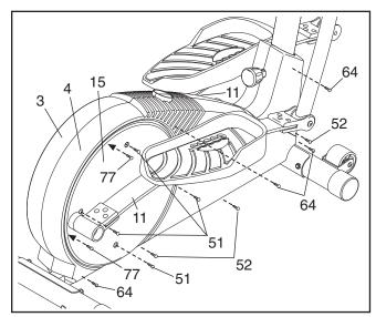
Next, remove the four Screws (51) from the right Pedal Disc (15), and slide the Pedal Disc off. Remove all Screws (52, 64) from the Right Side Shield (4) and the two Screws (77) from beneath the Pedal Disc, and remove the Right Side Shield. Remove all Screws (52) from the Left Side Shield (3) and remove the Left Side Shield.
