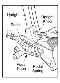
To adjust the upright, first turn the upright knob counterclockwise a few turns to loosen it. Next, pull the knob, raise or lower the upright to the desired height, and then release the knob. Move the upright up and down slightly until the pin on the knob snaps into one of the four adjustment holes in the upright. Make sure that the upright is not resting on top of the pin. Then, turn the knob clockwise until it is tight.
