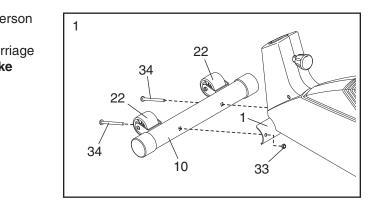
Identify the Front Stabiliser (10). Whilst another person lifts the front of the Frame (1), attach the Front Stabiliser to the Frame with two M10 x 75mm Carriage Bolts (34) and two M10 Nylon Locknuts (33). Make sure that the Front Stabiliser is turned so the Wheels (22) are not touching the floor.
