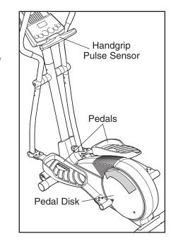
that you move the pedal disks in the direction shown by the arrow; however, for variety, you may turn the pedal disks in the opposite direction.
