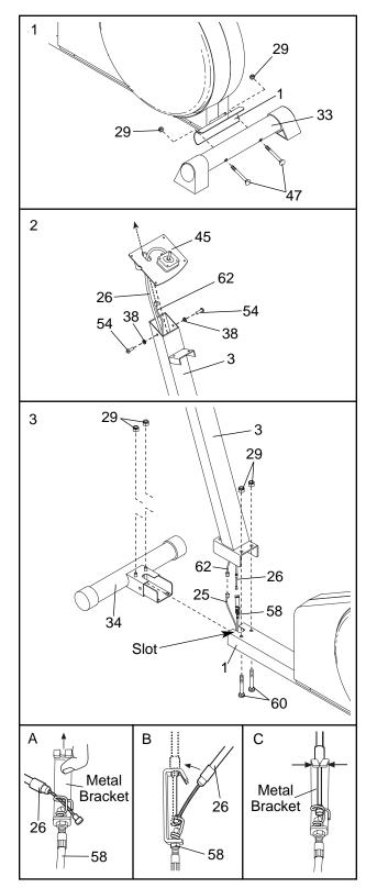
While a second person holds the Console (6) near the Console Bracket (45), connect the Extension Wire (62) to the console wire. Make sure the slack Resistance Cable (26) is pulled out of the Upright (3).
