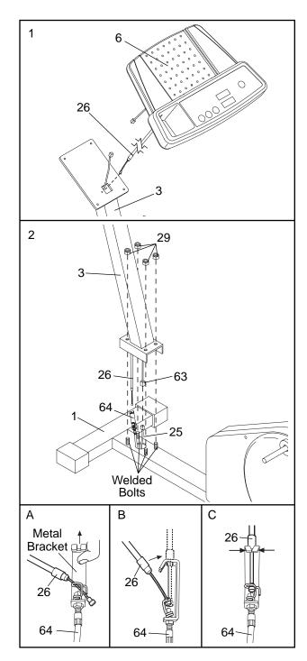
3. While another person holds the Console (6) near the Upright (3), connect the console wire to the Extension Wire (63).
