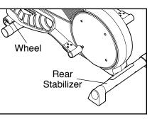
until it can be moved on the front wheels. Carefully move the elliptical crosstrainer to the desired location and then lower it. **CAUTION: To decrease the possibility of injury, bend your legs and keep your back straight as you lift the rear stabilizer; make sure to lift with your legs rather than your back.**
