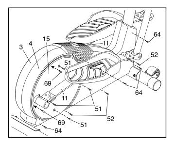
Next, remove the four Screws (51) from the right Pedal Disc (15), and slide the Pedal Disc off. Remove all Screws (52, 64) from the Right Side Shield (4) and the two Screws (69) from beneath the Pedal Disc, and remove the Right Side Shield (4). Remove all Screws (52) from the Left Side Shield (3) and remove the Left Side Shield.
