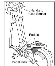
either direction. It is recommended that you move the pedal disks in the direction shown by the arrow; however, for variety, you may turn the pedal disks in the opposite direction.
