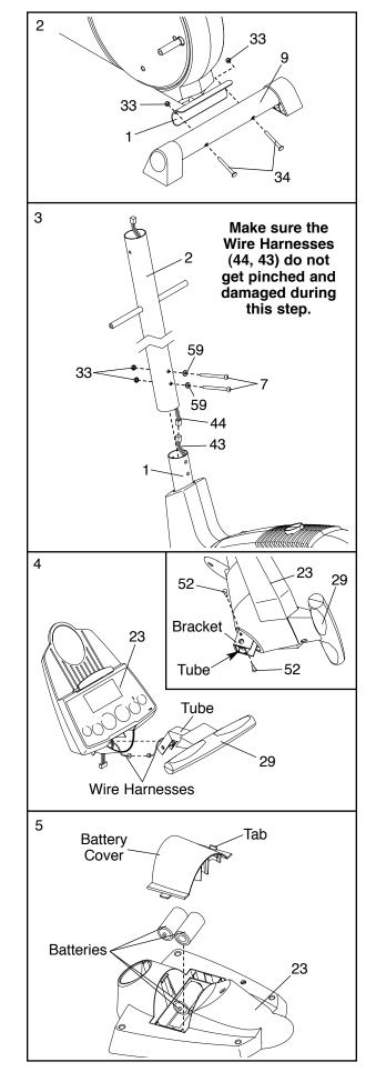
6. While another person holds the Console (23) in the position shown, connect the wire harness on the Console to the Extension Wire Harness (44). Insert the excess wire harness into the Upright (2).
