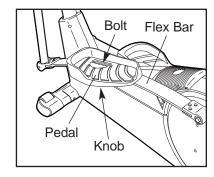
pedal forward or backward to the desired position, and then retighten the knob. Make sure that both pedals are in the same position.
