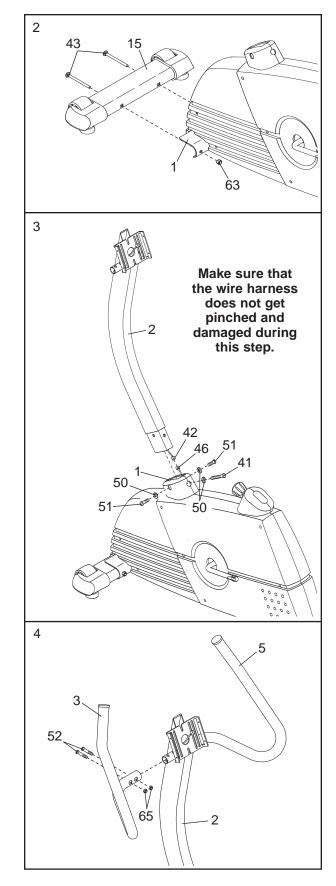
While another person holds the Upright (2) in the position shown, connect the Upper Wire Harness (42) to the Reed Switch Wire (46). Gently pull the upper end of the Upper Wire Harness to remove any slack.
