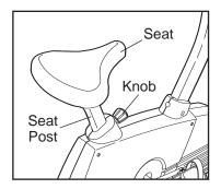
seat, first turn the seat knob counterclockwise two or three turns to loosen it (if the seat knob is not loosened enough, it may scratch the seat post). Next, pull the knob, slide the seat post to the desired height, and then release the knob. **Move the seat post up and down slightly until the pin on the knob snaps into one of the holes in the seat post.** Then, turn the knob clockwise until it is tight.
