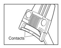
the handgrip pulse sensor, with your palms on the contacts closest to you and your fingers touching the contacts on the opposite side of the handgrip pulse sensor. **Avoid moving your hands.** When your pulse is detected, the heart-shaped indicator in the upper part of the display will begin to flash each time your heart beats. After a moment your heart rate will be shown.
