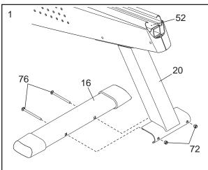
2. Orient the Front Stabilizer (15) as shown. While another person lifts the front of the Frame (1), attach the Front Stabilizer to the Frame with two M10 x 112mm Carriage Bolts (76) and two M10 Nylon Locknuts (72).
