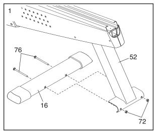
Orient the Front Stabilizer (15) as shown. While another person lifts the front of the Frame (1), attach the Front Stabilizer to the Frame with two M10 x 112mm Carriage Bolts (76) and two M10 Nylon Locknuts (72).
