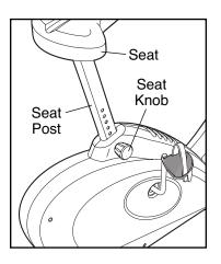
loosen it (if the knob is not loosened enough, it may scratch the seat post). Next, pull the knob, slide the seat post to the desired height, and then release the knob. Move the seat post upward and downward slightly until the pin on the knob snaps into one of the holes in the seat post. Then, turn the knob clockwise until it is tight.
