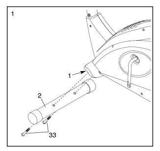
2. While another person lifts the rear of the Frame (1), attach the Rear Stabilizer (14) to the Frame with two M10 x 74mm Button Screws (33).
