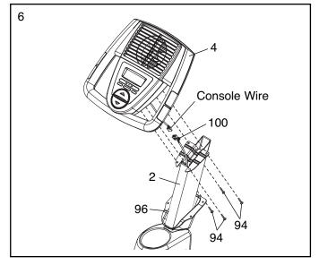
7. Slide the Console Cover (96) (see the drawing in step 6) upward to the Console (4). Attach the Console Cover with two M4 x 16mm Screws (84).
