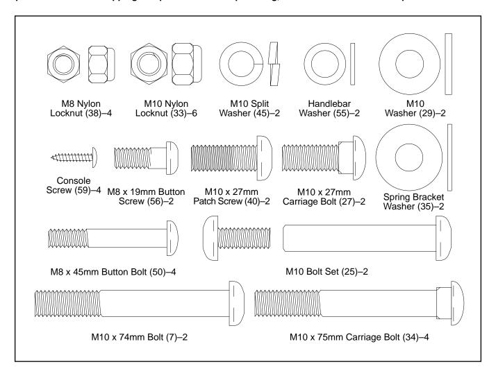
Identify the Front Stabilizer (10), which has round Endcaps (21) on it. While another person lifts the front of the Frame (1), attach the Front Stabilizer to the Frame with two M10 x 75mm Carriage Bolts (34) and two M10 Nylon Locknuts (33).
