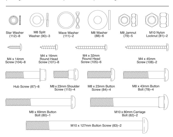
1. While another person lifts the Base (1), attach the Front Stabilizer (6) to the Base with two M10 x 80mm Carriage Bolts (82) and two M10 Nylon Locknuts (81).
