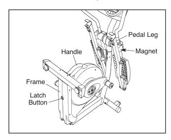
To use the elliptical exerciser, first hold the handle, press the latch button, and lower the frame.
