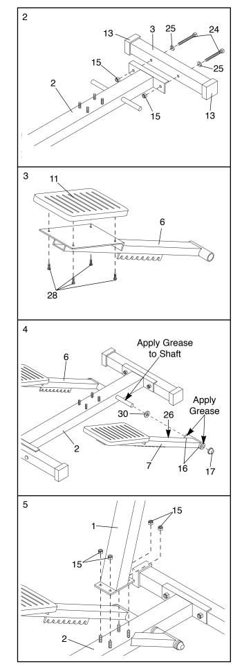
6. Apply grease to the shafts on the Upright (1).
