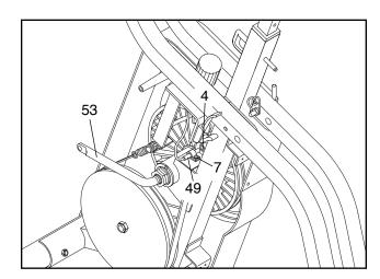
Next, locate the Reed Switch (49). Turn the Crank (53) until the Magnet (4) is aligned with the Reed Switch. Loosen but do not remove the M4 x 16mm Screw (7). Slide the Reed Switch slightly closer to or away from the Magnet. Retighten the Screw. Turn the Crank for a moment. Repeat until the console displays correct feedback. When the Reed Switch is correctly adjusted, reattach the left side shield and pedal.
