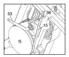
**fully** close the Strap Clamp. Turn the Crank (53) for a moment to make sure that there is not too much resistance. When the Resistance Strap is properly adjusted, reattach the left side shield and pedal.
