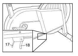
end of the Resistance Strap (17) and pull it back **slightly** to remove any slack. While holding the end of the Resistance Strap, **fully** close the Strap Buckle. Turn the crank for a moment to make sure that there is not too much resistance.
