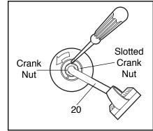
screwdriver in one of the slots in the slotted crank nut. Lightly tap the screwdriver with a hammer to turn the slotted crank nut counterclockwise until the arms are no longer loose. **Do not overtighten the slotted crank nut.** When the slotted crank nut is properly tightened, retighten the Crank Nut.
