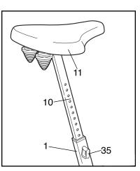
remove the Seat Pin (35). Align one of the holes in the Seat Post (10) with the hole in the Frame (1). Insert the Seat Pin into the Frame and the Seat Post. Caution: Make sure to insert the Seat Pin through one of the holes in the Seat Post; do not insert the Seat Pin under the Seat Post.
