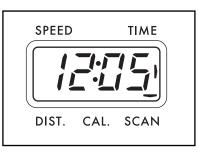
a flashing mode indicator will show which mode is currently displayed. Note: If a different mode is selected, you can select the scan mode again by repeatedly pressing the mode button. Speed, time, distance or calorie mode— To select one of these modes for continuous display, press the mode button repeatedly. The mode indicators
