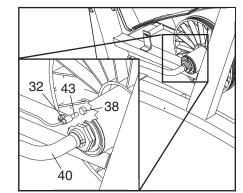
indicated M4 x 16mm Screw (32). Slide the Reed Switch slightly closer to or away from the Magnet, and then retighten the Screw. Turn the Crank Arm for a moment. Repeat until the console displays correct feedback. When the Reed Switch is correctly adjusted, reattach the left side shield, the side shield cover, and the left pedal.
