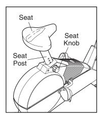
loosen it (if the knob is not loosened enough, it may scratch the seat post). Next, pull the knob, slide the seat post to the desired height, and then release the knob. **Move the seat post up and down slightly until the pin on the knob snaps into one of the holes in the seat post.** Then, turn the knob clockwise until it is tight.
