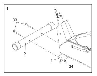
2. While another person lifts the back of the Frame (1) slightly, attach the Rear Stabilizer (30) to the Frame with two M10 x 75mm Carriage Bolts (33) and two M10 Black Nylon Locknuts (34).
