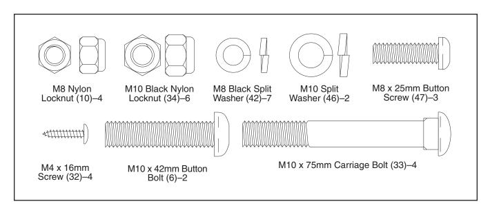
Identify the Front Stabilizer (2). While another person lifts the front of the Frame (1) slightly, attach the Front Stabilizer to the Frame with two M10 x 75mm Carriage Bolts (33) and two M10 Black Nylon Locknuts (34).
