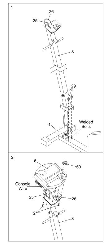
While another person holds the Console (6) near the Upright (3), connect the console wire to the Sensor Wire (25).
