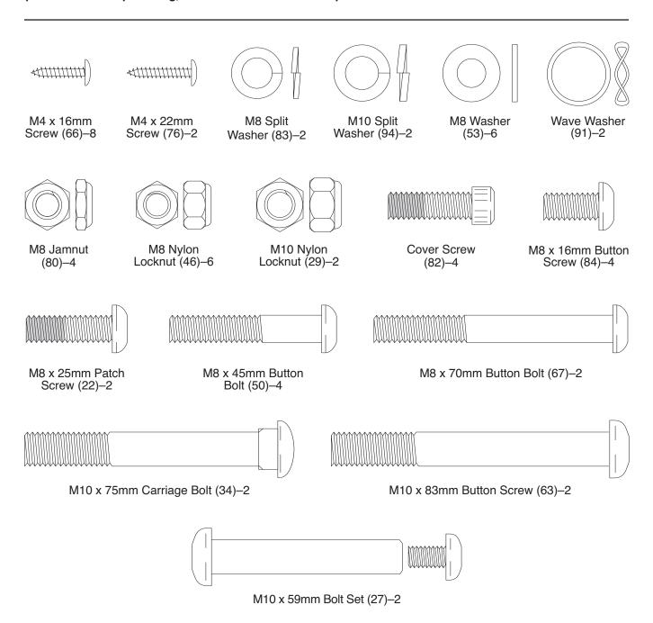
Identify the Rear Stabilizer (4). While another person lifts the rear of the Frame (1), attach the Rear Stabilizer to the Frame with two M10 x 75mm Carriage Bolts (34) and two M10 Nylon Locknuts (29).
