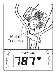
handgrips too tightly; excessive movement or pressure may interfere with heart rate readings. When your pulse is detected, the heart-shaped indicator in the center display will flash each time your heart beats, and your heart rate will be shown.
