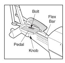
upward, slide the pedal forward or backward to the desired position, and then retighten the knob. Make sure that both pedals are in the same position.
