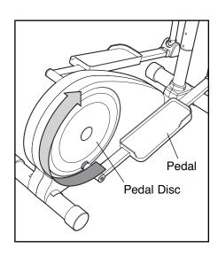
motion. Note: The pedal discs can turn in either direction. It is recommended that you turn the pedal discs in the direction shown above; however, for variety, you can turn the pedal discs in the opposite direction.
