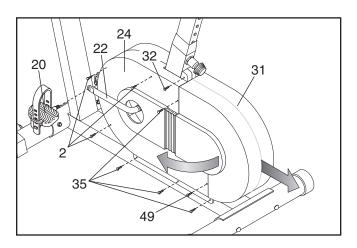
Next, locate the Reed Switch (4). Turn the arms of the Crank (22) until the Magnet (33) is aligned with the Reed Switch. Loosen but do not remove the indicated Screw (35). Slide the Reed Switch slightly closer to or away from the Magnet. Retighten the Screw. Turn the Crank for a moment. Repeat until the console displays correct feedback. When the Reed Switch is correctly adjusted, reattach the left side shield, flywheel cover and left pedal.
