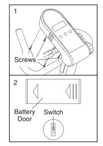
(see drawing 1). Lift the console a few inches and turn it over, being careful not to pull on the wires. Next, look into the hole below the battery door, and locate the small switch (see drawing 2). (Note: It may be necessary to look into the hole and to the left side to find the small switch.) Slide the switch up or down to change the unit of measurement. Reattach the console with the four screws.
