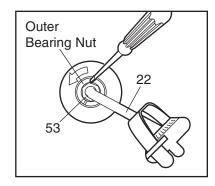
screwdriver in one of the slots in the outer bearing nut. Tap the screwdriver with a hammer to turn the outer bearing nut counterclockwise until the arms are no longer loose. **Do not overtighten the outer bearing nut.** When the outer bearing nut is properly tightened, retighten the Hex Jam Nut. The scan mode— Repeatedly press the mode button until an arrow appears under the scan symbol. When the scan mode is
