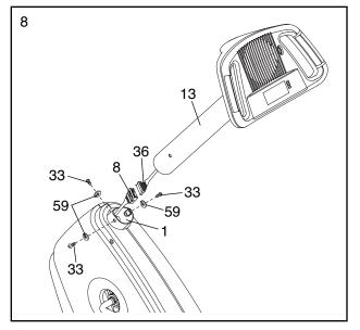
Identify the Left Pedal (24), which is marked with an "L." Using an adjustable wrench, firmly tighten the Left Pedal *counterclockwise* into the left arm of the Crank (31). Tighten the Right Pedal (not shown) *clockwise* into the right arm of the Crank. IMPOR-TANT: Tighten both Pedals as firmly as possible. After using the exercise cycle for one week, retighten the Pedals. For best performance, the Pedals must be kept tightened.
