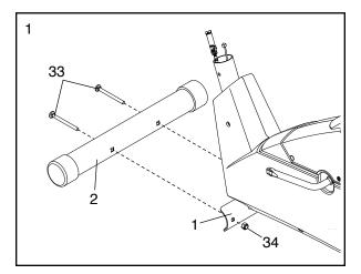
2. While another person lifts the back of the Frame (1) slightly, attach the Rear Stabilizer (30) to the Frame with two M10 x 75mm Carriage Bolts (33) and two M10 Black Nylon Locknuts (34).
