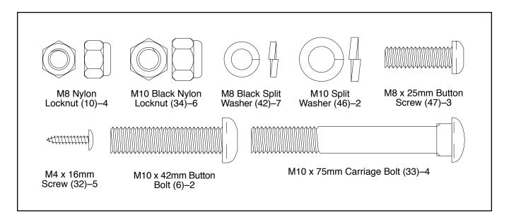
1. Identify the Front Stabilizer (2). While another person lifts the front of the Frame (1) slightly, attach the Front Stabilizer to the Frame with two M10 x 75mm Carriage Bolts (33) and two M10 Black Nylon Locknuts (34).
