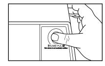
ed—fully press it down. Do not press too hard, or the circulation in your thumb will be restricted, and your pulse will not be detected. Next, raise your thumb slightly until the heart-shaped indicator in the right display flashes **steadily**. Hold your
