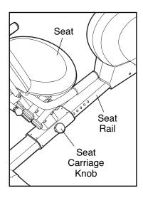
knob is not loosened enough, it may scratch the seat rail). Next, pull the knob, slide the seat carriage forward or backward to the desired position, and then release the knob into an adjustment hole in the seat rail. Then, turn the knob clockwise until it is tight. Make sure the seat carriage knob is engaged in an adjustment hole.
