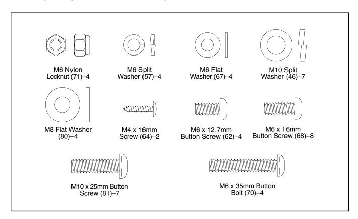
1. Attach the Rear Stabilizer (8) to the Frame (1) with four M10 x 25mm Button Screws (81) and four M10 Split Washers (46).
