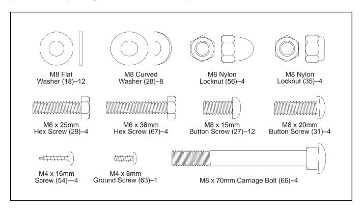
Identify the Front Stabilizer (2), which is shorter than the Rear Stabilizer (not shown). Attach the Front Stabilizer to the front of the Frame (1) with two M8 x 70mm Carriage Bolts (66), two M8 Curved Washers (28), and two M8 Acorn Nuts (56).
