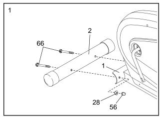
2. Attach the Rear Stabilizer (3) to the Rear Frame (44) with two M8 x 70mm Carriage Bolts (66), two M8 Curved Washers (28), and two M8 Acorn Nuts (56).
