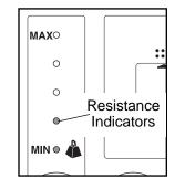
level 1 is selected; when the lowest indicator is brightly lit, resistance level 2 is selected; when the second indicator is dimly lit, resistance level 3 is selected; when the second indicator is brightly lit, resistance level 4 is selected; and so forth. When the highest indicator is brightly lit, resistance level 10, the most difficult level, is selected.
