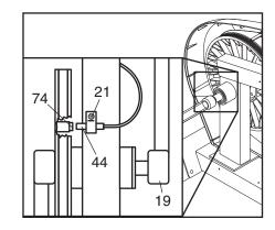
indicated M4 x 16mm Screw (21). Slide the Reed Switch slightly closer to or away from the Magnet. Then, retighten the Screw. Turn the Crank for a moment. Repeat until the console displays correct feedback. When the Reed Switch is correctly adjusted, reattach the left side shield and the left pedal.
