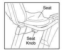
adjust the seat, make sure that your knees will not touch the handlebar or the console when you pedal. To adjust the seat, first turn the seat knob counterclockwise two or three turns to loosen it (if the seat knob is not loosened enough, it may scratch the frame). Next, pull the seat knob, slide the seat to the desired position, and then release the seat knob. Make sure to move the seat back and forth slightly until it locks in position. Then, turn the seat knob
