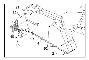
Using an adjustable wrench, turn the Left Pedal (40) clockwise and remove it from the Crank (19). Next, remove the two M4 x 16mm Screws (21) and the five M4 x 38mm Screws (62) from the Left Side Shield (4). Make sure that the left arm of the Crank is in the position shown above and carefully slide the Left Side Shield forward off the arm of the Crank.
