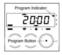
manual mode, press the program button until the program indicator disappears. The programs will be selected in the following order: program 1 (Interval), program 2 (Aerobic), program 3 (Fat Burn), manual mode.
