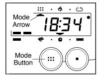
scan mode is selected, the console will display the speed, time, distance, lap, and calorie modes, for 5 seconds each, in a repeating cycle.
