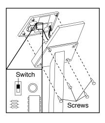
to change the unit of measurement. Remove the batteries for a few seconds and then put them back in. Reattach the console with the four screws. **Be careful not to pinch any of the wires.**
