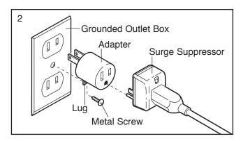
This product is for use on a nominal 120-volt circuit, and has a grounding plug that looks like the plug illustrated in drawing 1. A temporary adapter that looks like the adapter illustrated in drawing 2 may be used to connect the surge suppressor to a 2-pole receptacle as shown in drawing 2 if a properly grounded outlet is not available.
