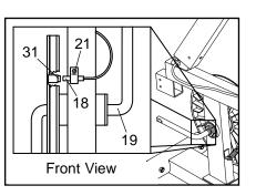
remove the M4 x 16mm Screw (21). Slide the Reed Switch slightly closer to or away from the Magnet. Retighten the Screw. Turn the Crank for a moment. Repeat until the console displays correct feedback. When the Reed Switch is correctly adjusted, reattach the left side shield and the pedal.
