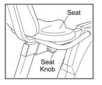
the seat knob counterclockwise to loosen it (if the seat knob is not loosened enough, it may scratch the frame). Next, slide the seat to the desired position, and then retighten the seat knob. **IMPORTANT: After you adjust the seat, make sure that your knees will not touch the handlebar or the console when you pedal.**
