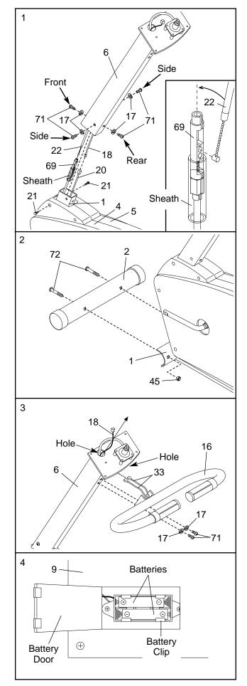
5. Hold the Console (9) near the Upright (6) as shown. Identify the green console ground wire and attach it to the Upright with an M4 x 16mm Screw (21).
