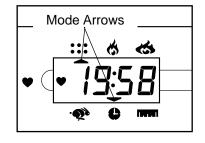
flashing mode arrow will show which mode is currently displayed. Note: If a different mode is selected, you can select the scan mode again by repeatedly pressing the mode button.
