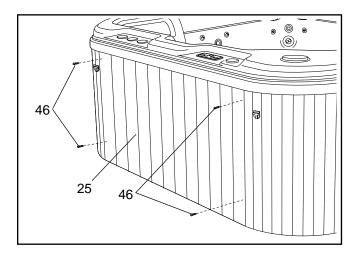
To replace the Access Panel, hold the Access Panel in place and secure it with the four #10 x 2" Machine Screws (46). Be careful not to overtighten the Screws.
