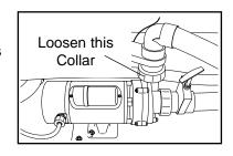
and air to escape from the pumps and related plumbing. Then, retighten the collars.
