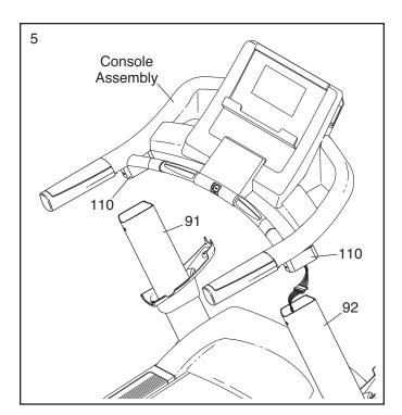
Partially tighten three 3/8" x 1 1/4" Bolts (2) with three 3/8" Star Washers (6) into the Right Upright (92); do not fully tighten the Bolts yet.
