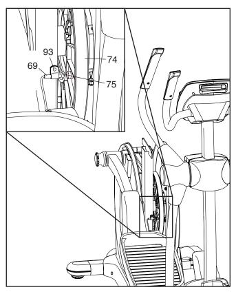
Next, rotate the Large Pulley (74) until a Magnet (75) is aligned with the Reed Switch (69). Slide the Reed Switch slightly toward or away from the Magnet. Then, retighten the M4 x 16mm Screw (93).
