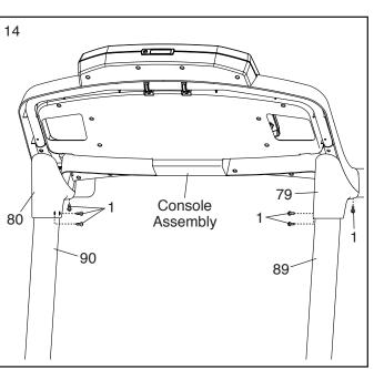
Attach the Left Tray (107) and the Right Tray (102) to the console assembly with four #8 x 1/2" Screws (1).
