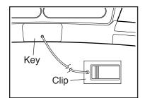
the console. After several seconds, the displays will light. **IMPORTANT: In an emergency, the key can be pulled from the console, causing the walking belt to slow to a stop. Test the clip by carefully taking a few steps backward; if the key is not pulled from the console, adjust the position of the clip.**
