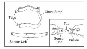
Next, wrap the chest pulse sensor around your chest and attach the other end of the chest strap to the sensor unit. Adjust the length of the chest strap, if necessary. The chest pulse
