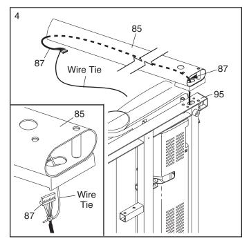
Hold the Right Upright (85) against the Base (95). Be careful not to pinch the Upright Wire (87). Insert two 3/8" x 4" Patch Bolts (7) and a 3/8" x 1 1/2" Patch Bolt (3) with three 3/8" Star Washers (11) into the Right Upright.
