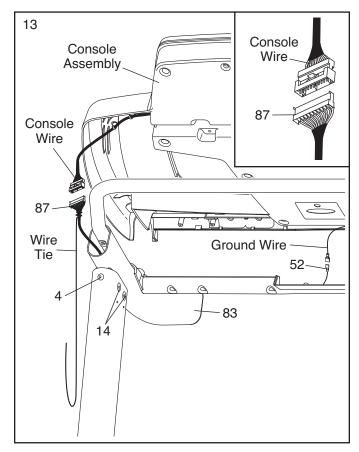
14. Set the console assembly on the Left and Right Handrails (82, 83). Be careful not to pinch any wires. Insert the excess Upright Wire (87) into the Right Handrail.
