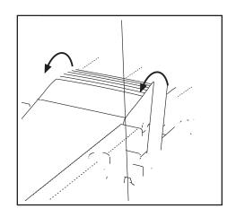
Locate the Reed Switch (63) and the Magnet (46) on the left side of the Pulley (47). Turn the Pulley until the Magnet is aligned with the Reed Switch. **Make sure that the gap between the Magnet and the Reed Switch is about 1/8".** If necessary, loosen the Screw (7), move the Reed Switch slightly, and then retighten the Screw. Reattach the Hood, and run the treadmill for a few minutes to check for a correct speed reading.
