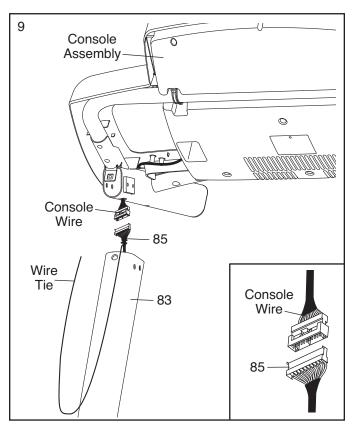
Set the console assembly on the Left and Right Uprights (82, 83). Be careful not to pinch any wires. Insert the excess wire into the Right Upright.
