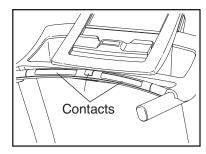
To measure your heart rate, stand on the foot rails and hold the contacts—avoid moving your hands. When your pulse is detected, your heart rate will be shown. For the most accurate heart rate reading, continue to hold the contacts for about 15 seconds.
