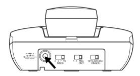
2. Plug the other end of the adapter into a standard AC outlet.
