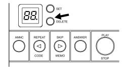
To erase all messages, while playback is stopped, hold down **DELETE**. The TAD sounds a long beep and 00 appears on the display.
