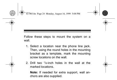
3. While holding the bracket against the wall, thread a screw through each hole, then tighten the screws.
