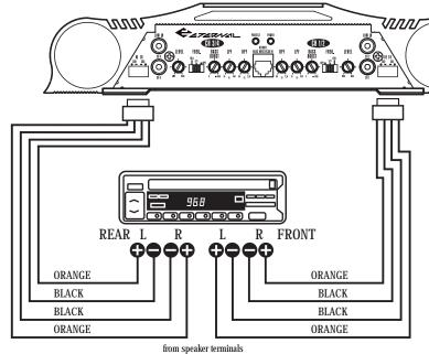
4 CH harness wiring for common ground connections
