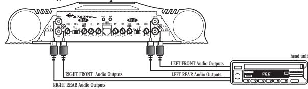
2 CHinput connections using low level inputs
