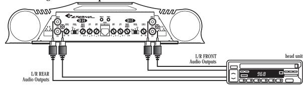
2 CHinput connections using low level inputs
