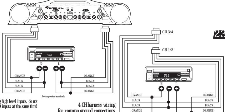
PIFASE NOIE If using high level inputs, do not use the low level RCA inputs at the same time!
