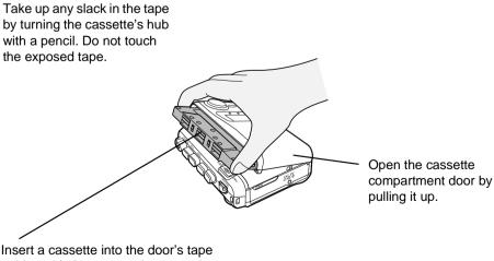
Insert a cassette into the door's tape guides with the cassette's open edge facing up, then close the door.
