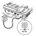
2. Route the adapter cable through the strain relief slot on the bottom of the telephone.
