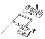
2. Plug one end of the supplied short modular cord into the **TEL LINE** jack on the back of the phone and plug the other end into a modular phone line jack. Then align the base's keyhole slots with the wall plate studs (or screws) and slide the base downward to secure it.
