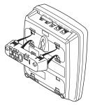
2. To connect the phone to a two-line phone jack, plug one end of the supplied long two-line modular cord into the TEL LINE 1/2 jack on the back of the phone. Route the cord through the strain-relief slot on the bracket.
